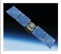
METEORITE is an ESPA Class Small Spacecraft Bus product family used for a variety of missions in LEO including High LEO (1000 to 1200 km). METEORITE is ideal for pathfinder constellation missions or other disaggregated mission types. METEORITE leverages the same core avionics from Moog's Space Vehicle family that have been demonstrated in missions from LEO to the Moon. The green propulsion system is ideal for rideshare or
